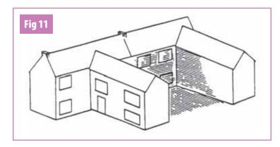
6.6 Finally, the 45 degree code deals only with daylight. Additional checks will need to be made for the sunlight which may be blocked. The windows of some existing buildings will also have rights to light. None of these guidelines here replace or necessarily satisfy the legal requirements contained in rights-to-light law.
