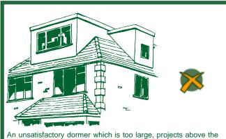
An unsatisfactory dormer which is too large, projects above the ridge, is on a hipped roof and wraps around more than one face of the roof.
