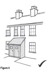
3.6 On semi-detached and terraced properties, it is particularly important to consider the symmetry and design of neighbouring porches (figure 4). A porch of poor design and quality that bears no relation to the symmetry of neighbouring properties or the terrace can damage the appearance of the whole street.
