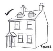
3.13 Dormer windows should not be higher than the existing ridgeline and should reflect the vertical lines, emphasis and positioning of existing doors and windows of your existing property (figures 8 and 9). The materials and window design should also match those of your original property. Please remember that the purpose of a dormer window is to provide light and not to gain increases in floor area.
