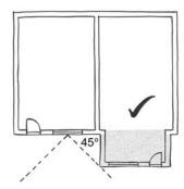
Figure 2 is an example where the 45-degree rule is applied. This two-storey extension is acceptable as it does not encroach within 45 degrees of the centre of a neighbouring property's window.
