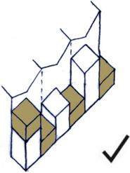
Particularly where there is existing variation in the rear elevations, extensions above existing rear projections will normally be acceptable providing they are visibly below the lowest point of the roof
