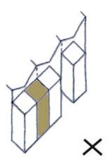
Where they project above upper ground floor level, rear infill extensions within the lightwell area can undermine the rhythm of the terrace
