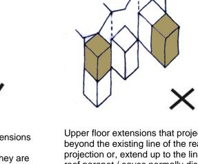
Upper floor extensions that project out beyond the existing line of the rear projection or, extend up to the line of the roof parapet / eaves normally disrupts the rhythm / unity of the terrace
