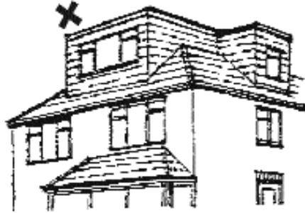
**dormer windows should be designed to match the style, alignment and proportions of existing windows.**
