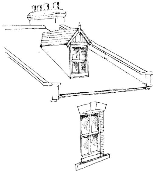
**loft conversions should use rooflights where possible to maintain the pitch of the roof and avoid overlooking**
