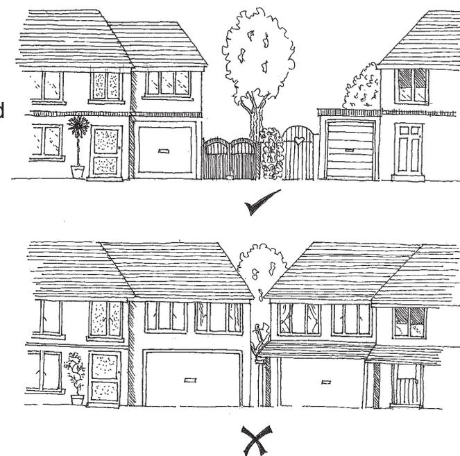
Fig. 8 -Two storey side extensions (the 'terracing' effect)
