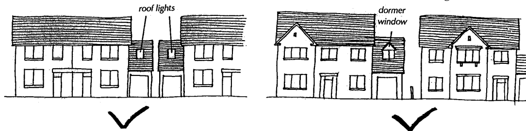
Fig.10 It may be possible to locate first floor accommodation within the roofspace of a side extension by use of dormer windows or roof lights so that it has the outward appearance of a single storey structure, and retains visual separation of dwellings.
