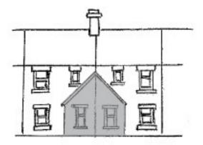
Flat roofed extensions rarely appear to blend harmoniously with the existing dwelling and are likely to present long term maintenance problems. Pitched roofs are preferable and should be to the same pitch as the main roof. If it is not possible to achieve a pitched roof to the same angle as the main house then this is a good indication that the size of the extension is not in keeping with the scale of the dwelling. Two storey extensions should always have pitched roofs.
