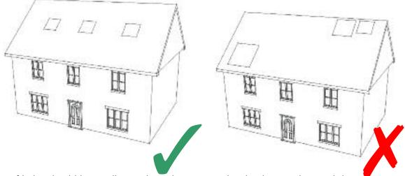
Roof lights should be small in scale and symmetrical with other window and door openings
