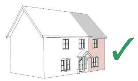
When adding an extension to the side of an end of terrace house it is sometimes more suitable to continue the terrace building line and roof ridge height. In this way the extension would appear as if it was originally designed to be part of the terrace, as one coherent building.
