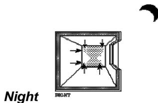
Figure 7 - Thermal mass in the interior absorbs heat from the sun and radiates the heat at night
