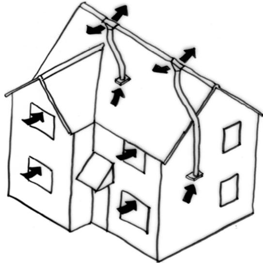
Fig 8 - Passive Stack Ventilation replaces the need for energy hungry extract fans.
