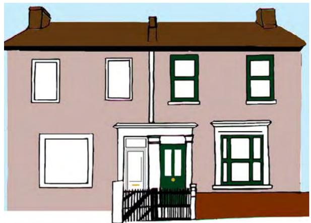
*Figure - 33 The original timber sash windows have been removed from the mid-nineteenth century house on the left and replaced by inappropriate window frames without glazing bars.*
