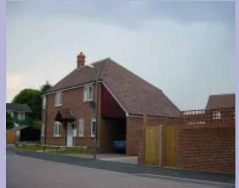
*This carport has been sensitively designed as the main roof has been extended at the same pitch to create it and uses the same roof tiles*
