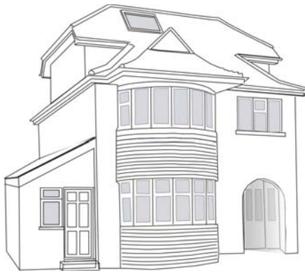
Figure 28: Dormers that alter and dominate the original roof form will not be supported.
